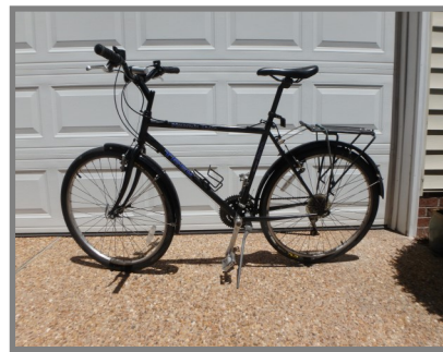
Hard tail mountain bikes make excellent city bikes when equipped w/fenders riser bars.
